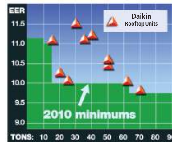
Maverick II rooftop systems are available with EERs that exceed ASHRAE 90.1-2007 requirements for the year 2010, which are approximately 6% more efficient than ASHRAE 90.1-2004 requirements.
